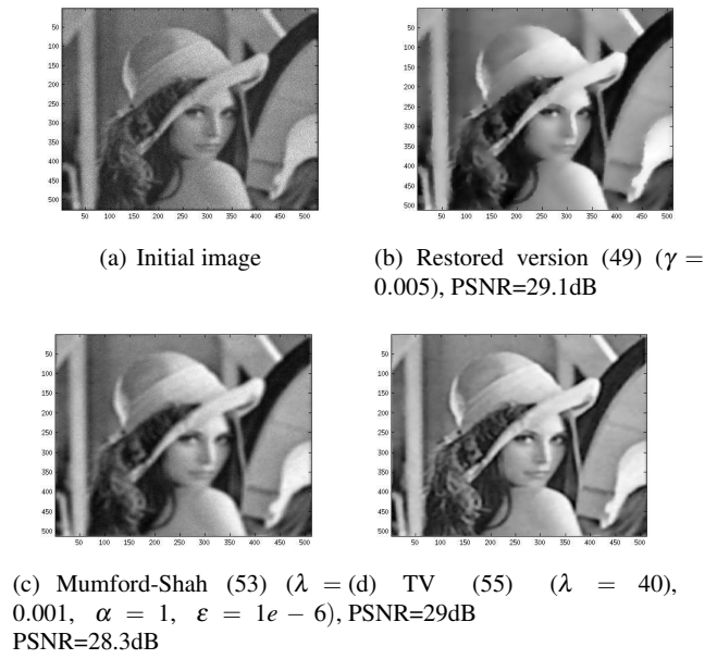
Fig. 15 Comparison of the restored versions for a Poissonian image blurred by Gaussian convolution ( \sigma = 3 )
