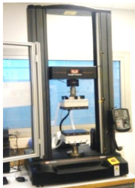
Figure 4: Press for sintering equipped with tow heating platens.
