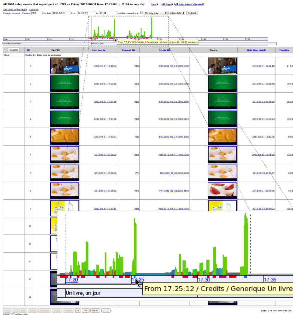
Fig. 3. A view on a 10-minute inter-programme: in that order: a teaser (1 st row); a set of commercials; a short 2-minutes literary programme (not in table, with its title sequence, starting 5 minutes late with respect to the electronic programme guide); a second set of commercials; a teaser; next programme title sequence. On the close-up are marked the already labelled sections, bright red for teasers, red for commercials, blue for credits/titles, cf. Table I.
