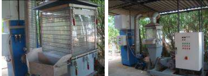
Figure 2 – AllJig S 400 ® jig used in the tests.
