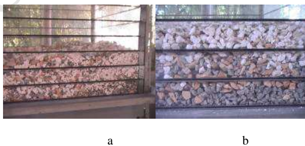
Figure 4 – (a) Beginning of the test with the particles having been mixed together; and (b) end of the test where it is clear that the particles have been stratified according to density.
