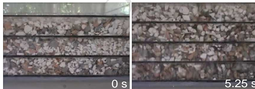
Figure 6. Observation of the particles distribution on the wall at the initial sorting time and at the maximum expansion 5.25 s.
