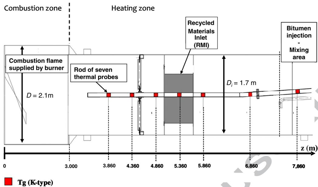
Figure 3 – Scheme of the rotary kiln set-up.
