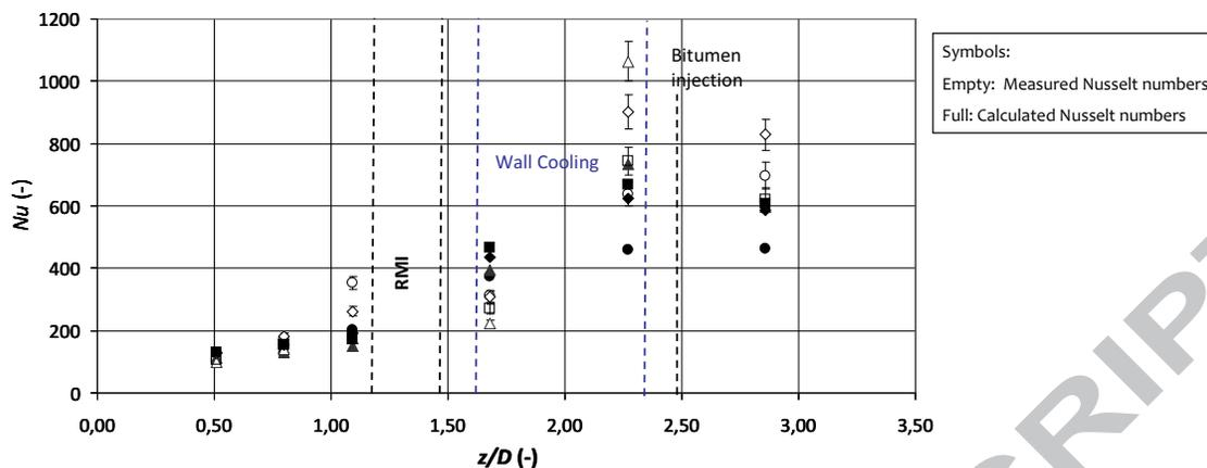
Figure 8 – Calculated and measured Nusselt numbers describing the inner parietal heat transfer in the heating zone measured in large-scale kiln at different aggregates feed rate {Circle :  $\dot{m}_a=26 \text{ kg.s}^{-1}$  - Triangle :  $\dot{m}_a=29 \text{ kg.s}^{-1}$  – Diamond :  $\dot{m}_a=31 \text{ kg.s}^{-1}$ - Square :  $\dot{m}_a=34 \text{ kg.s}^{-1}$ }.
