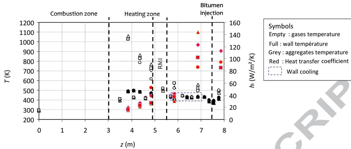
Figure 4 – Longitudinal temperatures and heat transfer coefficient measured in large-scale kiln at different aggregates feed rate { Circle :  $\dot{m}_a=26 \text{ kg.s}^{-1}$  - Triangle :  $\dot{m}_a=29 \text{ kg.s}^{-1}$  - Diamond :  $\dot{m}_a=31 \text{ kg.s}^{-1}$  - Square :  $\dot{m}_a=34 \text{ kg.s}^{-1}$  }.
