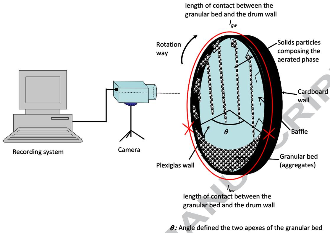
Figure 6 - Scheme of the visualization set-up.
