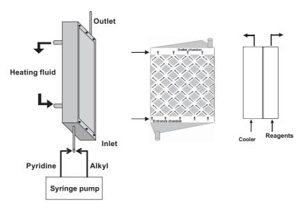
**Figure 2.** Left: Schematic representation of the heat exchanger/microstructured reactor:  $V = 10.2 \text{ cm}^3$ ,  $S/V = 24.6 \text{ cm}^{-1}$ . Middle: Schematic shape of microstructured reactor. Right: the plate reactor seen from the side.
