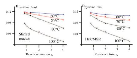
Figure 4. Conversion rate of [OcPy][Br] synthesis reaction at different temperatures against: reaction duration in stirred reactor (left) and residence time in Hex/MSR (right). n<sub>reagents</sub>: 0.126 mol
