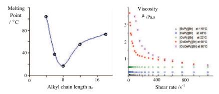
Figure 3. Left: Melting points of alkylpyridinium ILs against alkyl chain length; experimental uncertainty of ±2 °C. Right: Viscosity (measured at ILs melting point + 5 °C) dependency vs shear rate for various alkylpyridinium IL.
