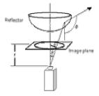
Figure 8: The panoramic vision system. The camera has a 640x480 pixels resolution and an equiangular mirror is used so that each pixel in the image covers the same view angle.
