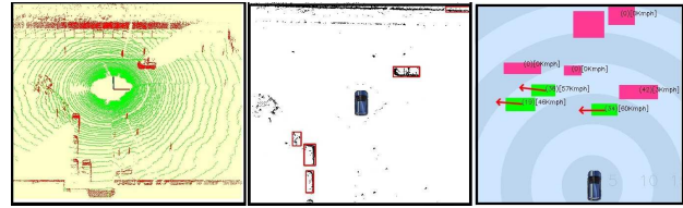
Fig. 8. Vehicle Tracking Results: Segmented point clouds (left), detected vehicles (middle), tracked vehicles (right)
