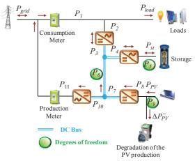
Fig. 1: Considered microgrid and power flows
