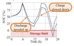
Fig. 2: SOC constraint violation with the fine model
