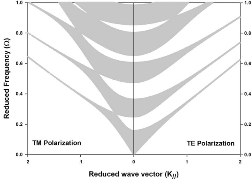
**Figure 2.** Projected band structure of the superlattice with thicknesses  $d_1 = d_2 = 0.5D$  for TE (right panel) and TM (left panel) modes. The reduced frequency,  $\Omega = \omega D/2\pi c$ , is presented as a function of the reduced wave vector,  $k_{||}$ . The shaded and white areas correspond respectively to the minbands and minigaps of the superlattice.
