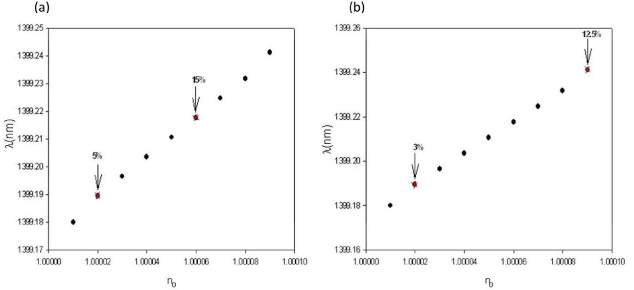
**Figure 7.** Resonant wavelength,  $\lambda$ , plotted as a function of polluted air highlighting two different concentrations of (a) methane in air and (b) ethane in air.
