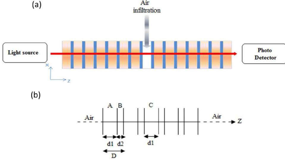
**Figure 1.** (a) Illustration of the photonic crystal sensor device used for the detection of a gas concentration. (b) Schematic representation of the stacked structure used for the calculation where A and B represent, respectively, the layers of magnesium fluoride ( $\text{MgF}_2$ ) and silicon (Si) and C represents the infiltrated gas to be sensed.
