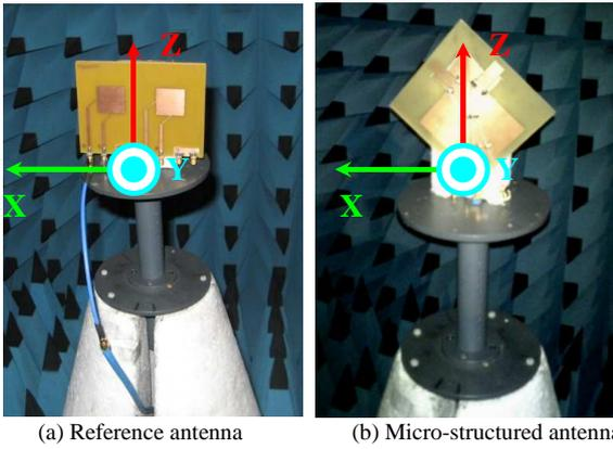
Fig. 4. Antenna array measurement and associated coordinated system.
