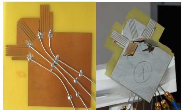
Fig. 2. Four ports and eight ports micro-structured antenna .
