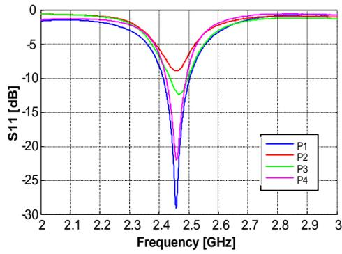
Fig. 3. Reflection coefficient of the micro-structured antenna array.
