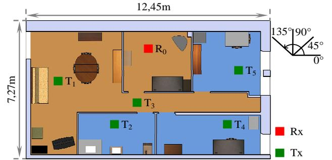
Fig. 10. Indoor environment with transmitter and receiver locations
