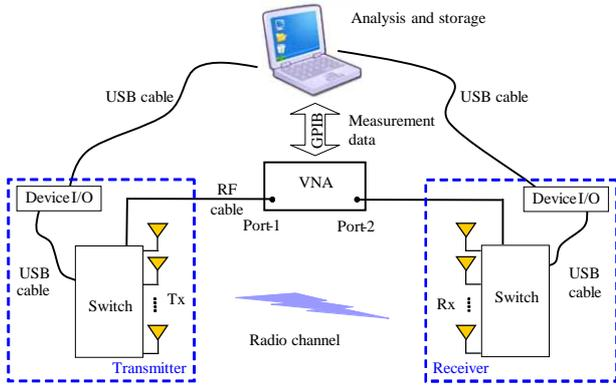
Fig. 9. Set-up of the MIMO channel sounder.
