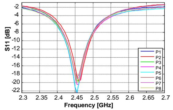
Fig. 7. Reflection Coefficient of the reference antenna array.
