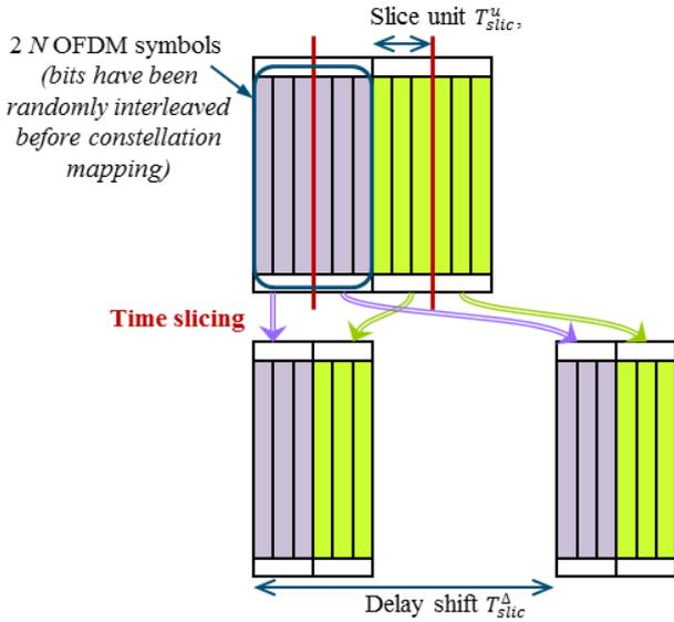
Fig. 9: Proposed time slicing principle (terrestrial link).
