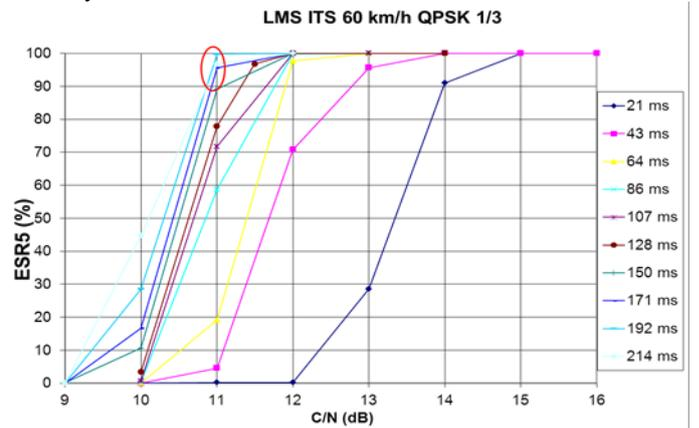
Fig. 11: Satellite case simulations results, LMS ITS channel.
