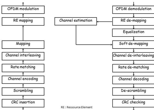
Fig. 13: Functional diagram of the CPHY platform.
