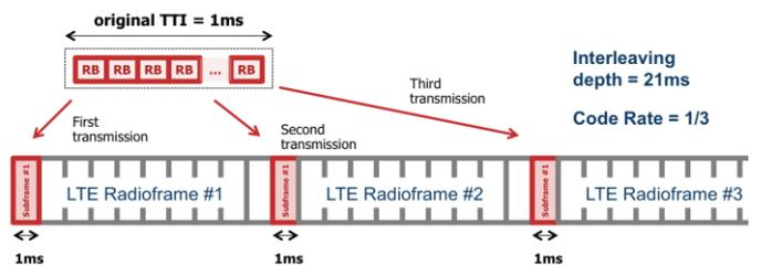
Fig. 6: Time interleaving based on automatic retransmissions.
