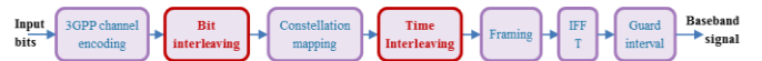
Fig. 8: Introduction of new interleaving blocks (in red) into the LTE transmission chain (terrestrial link).
