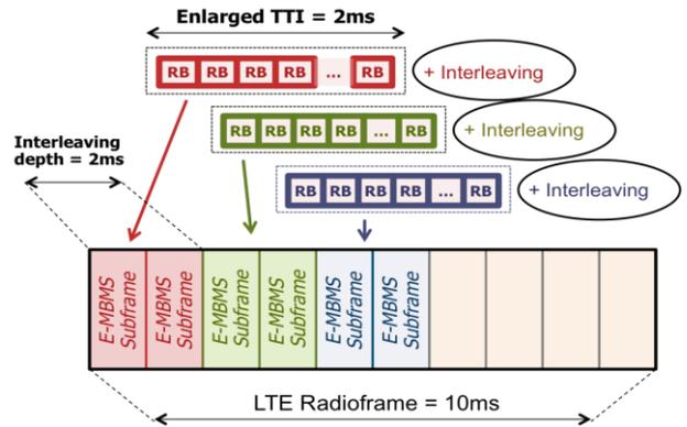
Fig. 4: Intra-frame interleaving and TTI enlargement of 2 ms.
