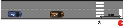
Fig. 5: Scenario chosen for the evaluation of the application for ADAS. Two vehicles (the subject vehicle V1 in blue, the leading vehicle V2 in orange), a pedestrian, a pedestrian crossing and a stop intersection.
