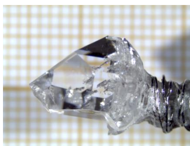
Figure 1. Picture of an \alpha -GeO 2 single crystal grown by the top seeded solution growth (TSSG) technique in K 2 Mo 4 O 13 flux.
