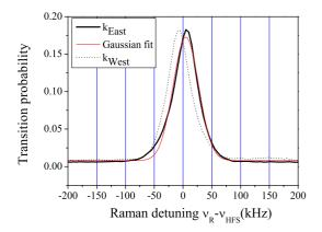
FIG. 13: Transition probability versus the detuning between the horizontal Raman lasers. Thick line: Raman spectrum with a momentum kick directed towards the East, thin line: a gaussian fit to the  $k_{East}$  spectrum. Dotted line: momentum kick towards the West.
