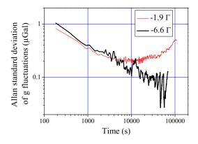
FIG. 9: Allan standard deviations of gravity fluctuations, calculated from the mean values of the effective velocity distributions, at detunings  $-1.9\Gamma$  (thin line) and  $-6.6\Gamma$  (thick line).
