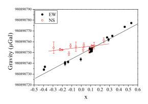
FIG. 1: Gravity measurement as a function of the intensity unbalance between molasses beams along the EW and NS directions. The detuning of the first molasses phase is  $-1.9\Gamma$ .
