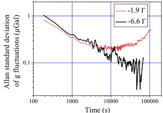
FIG. 9: Allan standard deviations of gravity fluctuations, calculated from the mean values of the effective velocity distributions, at detunings  $-1.9\Gamma$  (thin line) and  $-6.6\Gamma$  (thick line).
