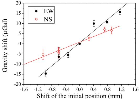
FIG. 4: Gravity shift as a function of the shift of the atoms from the initial position, for displacements in the EW and NS directions.
