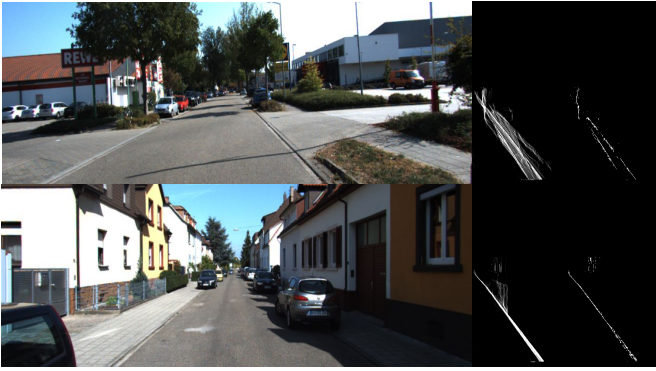
Figure 4. Examples of v -disparity map in different situations (selected from UU dataset in KITTI-ROAD). Up left : Image of which stereo baseline is not parallel to the ground plane. Bottom left : Image taken from common situation. Middle: v -disparity maps generated from pre-detected ROI. Right: refined v -disparity with high intensity pixels preserved.
