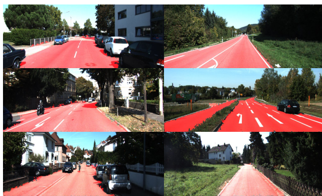
Figure 3. Binary map detection results on the KITTI-ROAD dataset. Each line presents two images from UM, UMM and UU dataset separately.
