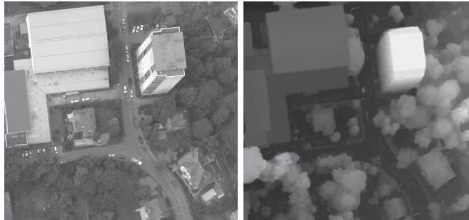
Fig. 12: Estimated depth map (right) for a large aerial stereo data set of Graz using the primal-dual approach in [130]. One of the images of the corresponding stereoscopic pair (of size 1500 \times 1400 ) is shown on the left.
