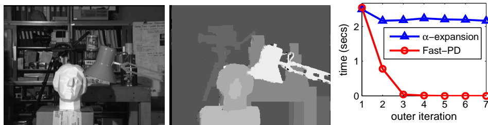
(b) 'Tsukuba' stereo matching (from left to right: left image, FastPD output, time comparison plot)
