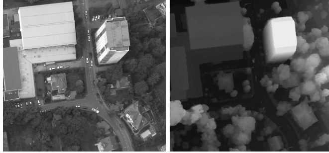
Fig. 11: Estimated depth map (right) for a large aerial stereo data set of Graz using the primal-dual approach in [117]. One of the images of the corresponding stereoscopic pair (of size 1500 \times 1400 ) is shown on the left.
