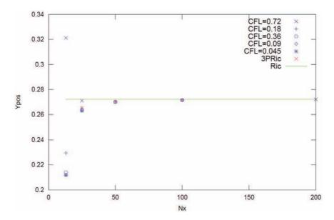
**Fig. 20.** Time evolution of the vertical position of the particle for various CFL numbers. The asymptotic numerical values 3PRic and Ric stands for extrapolation of  $Y_p$  through the Richardson theory [101] on 3 points (3PRic) and 4 points (Ric).
