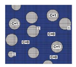
Fig. 1. Definition sketch of the fictitious domain approach for a finite size particulate flow. The underlaying grid, the phase function C and the fluid-particle interface  $\Sigma$  are plotted.
