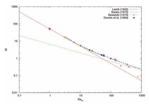
**Fig. 17.** Relation between the Reynolds number and the dimensionless torque. Lines correspond to references cited below. Symbols correspond to actual for different refinements (cross, circle and square for 10, 20 and 40 nodes per diameter). Colors (red, orange, yellow, green, blue, magenta and pink) are respectively for  $\mu = 10^{b}$ ,  $b = \{0, 0.5, ..., 3\}$ . (For interpretation of the references to color in this figure, the reader is referred to the web version of this article.)
