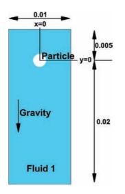
Fig. 9. Definition sketch of the settling of a cylindrical shape particle.
