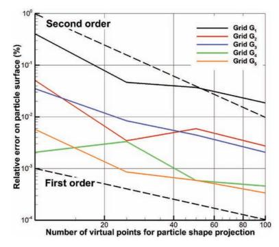
Fig. 6. Error on the projected surface of a circular shape particle according to the number of virtual points in each space direction and to the Eulerian grid used.
