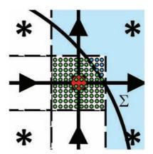
**Fig. 5.** Two-dimensional network of  $10^{Ndim}$  virtual points used to estimate the local solid fraction  $C^{n+1}$  thanks to a Lagrangian position  $\mathbf{X}^{l,L,n+1}$  of a particle, whose interface is noted  $\Sigma$ . In green are plotted the virtual points belonging to the particle and in blue the other ones. In the example,  $C^{n+1} = 92/100 = 0.92$ . (For interpretation of the references to color in this figure, the reader is referred to the web version of this article.)
