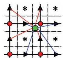
Fig. 4. Eulerian velocity kernel (u-components in blue and v-components in red) used in two dimensions to estimate the components of the interpolation Lagrangian velocity points (green point). (For interpretation of the references to color in this figure, the reader is referred to the web version of this article.)
