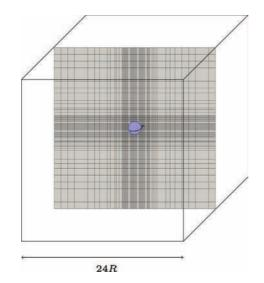
Fig. 14. Typical Eulerian grid used to simulate the rotation of a particle in a box with  $N_d = 20$ .
