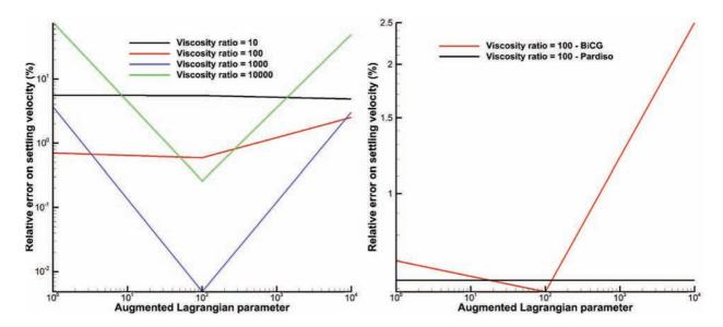
Fig. 10. Comparison of relative errors on settling velocity: left, results obtained with the iterative solver for various viscosity ratios and augmented Lagrangian parameter K and right, comparison of PARDISO and BiCGSTAB II for a viscosity ratio of 100.
