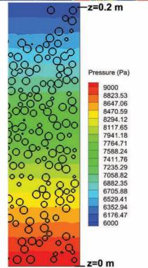
**Fig. 24.** Instantaneous view of the fluidized bed in a medium vertical slice at t = 10 s – top: particles and velocity field in a zoom – bottom: particles (lines) and pressure in the whole bed. (For interpretation of the references to color in this figure, the reader is referred to the web version of this article.)
