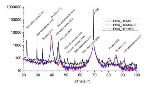
Figure 3. X-ray diffractogram (in  $\theta/2\theta$  configuration) of three Pt depositions on silicon between 20 and  $100^{\circ}$ .
