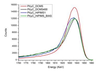
**Figure 2.** Rutherford Backscattering Spectroscopy spectrum between 1760 and 1860 keV (corresponding to the platinum peak) of the four Pt depositions on microporous carbon (GDL 10BC Sigracet®). The Pt loadings corresponding to the areas under the four peaks were measured (20 μgPt.cm-2 for each). The kinetic energy of the 4He particles and the scattering angle are fixed to 2 MeV and 165°, respectively.
