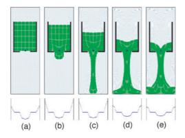
**Fig. 1.** Snapshots of the model. (a) Initial conditions, (b)  $t = 4.75 \cdot 10^{-4} \text{ sec.}$ , (c)  $t = 1.42 \cdot 10^{-3} \text{ sec.}$ , (d)  $t = 2.85 \cdot 10^{-3} \text{ sec.}$  and (e)  $t = 3.8 \cdot 10^{-3} \text{ sec.}$
