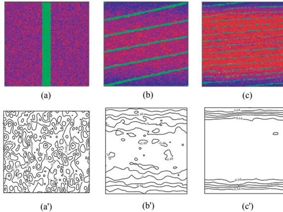
**Fig. 4.** (a) Initial conditions with random particle orientation, (b) beginning of the anisotropic behaviour and (c) the material is oriented. Plots (a'), (b') and (c') are the isovals of the director orientation respectively corresponding to configuration (a), (b) and (c)
