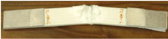
Fig. 6. 0° Tensile specimen broken.
