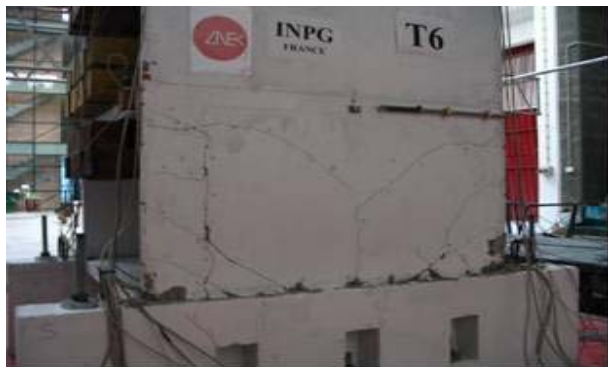
Figure 19. Experimental damage pattern for T6 motion
