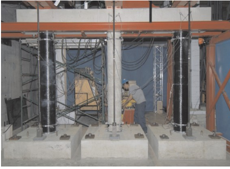
Figure 3. Bridge pier mockup with partial retrofitting.
