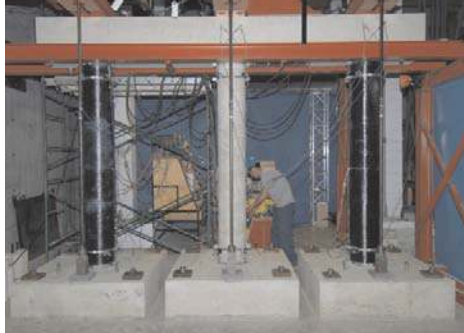
Figure 3. Bridge pier mockup with partial retrofitting.
