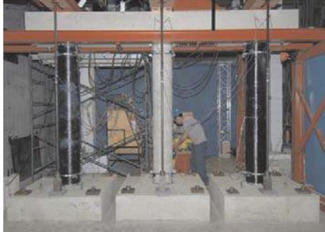
Figure 3. Bridge pier mockup with partial retrofitting.
