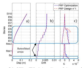
**Figure 5.6.** GCH - FRP design  $n^{\circ}1$  retrofitting: retrofitted Vs non-retrofitted configuration. Response of one pier: (a) displacements, (b) inter-story drifts, (c) steel strains.
