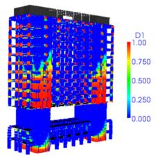
**Figure 4.3.** GCH – Distribution of  $D_1$  (tension damage).
