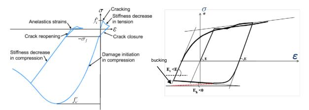
**Figure 3.2.** La Borderie model - uniaxial stress-strain relation.
