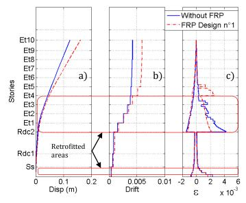
**Figure 5.4.** GCH (FRP design  $n^{\circ}1$ ) - retrofitted Vs non-retrofitted configuration. Response of one pier: (a) displacements, (b) inter-story drifts, (c) steel strains.
