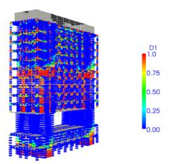
**Figure 5.5.** GCH – FRP retrofitting - design  $n^{\circ}1$  - Distribution of  $D_1$  (tension damage).
