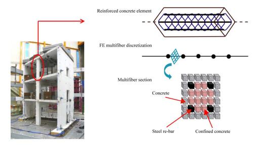
Figure 3.1. Multifiber beam modeling
