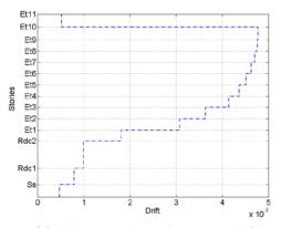
**Figure 4.2.** GCH - Maximum inter-story drift in one pier: (X) longitudinal and (Y) transverse direction.
