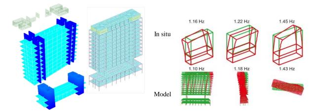
Figure 3.4. CGH – Finite element mesh.
