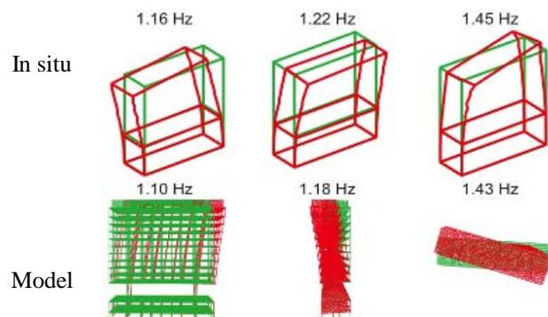
**Figure 3.5.** GCH – Modal analysis – In-situ records Vs model.
