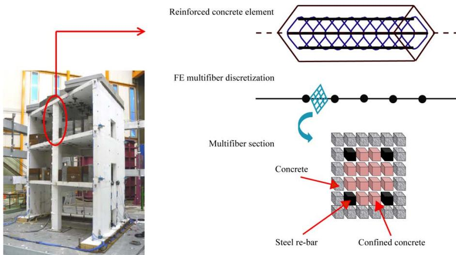
**Figure 3.1.** Multifiber beam modeling
