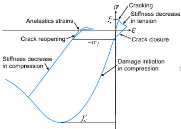
**Figure 3.2.** La Borderie model - uniaxial stress-strain relation.
