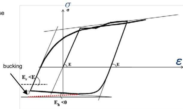
**Figure 3.3.** Menegotto & Pinto model - uniaxial stress-strain relation.
