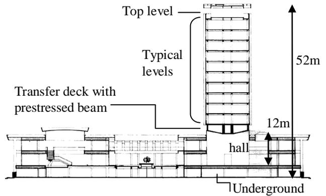
**Figure 2.2.** GCH - Transverse view of the structure
