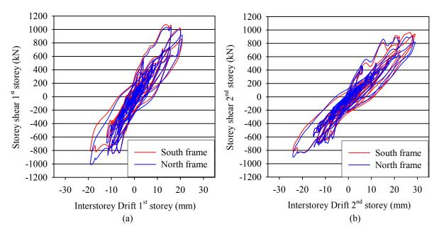
Figure 3.3. Experiment at 0.25 g acceleration (a) 1<sup>st</sup> storey interstorey drift, (b) 2<sup>nd</sup> storey interstorey drift
