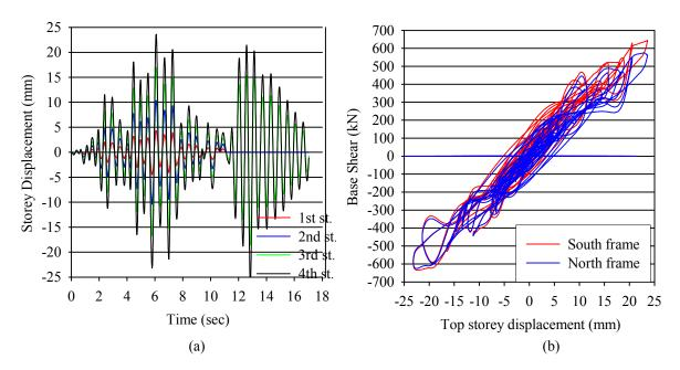
**Figure 3.1.** Experiment at 0.10 g acceleration (a) Variation of the storey displacements with time, (b) Base shear versus top storey displacement for the north and south frames
