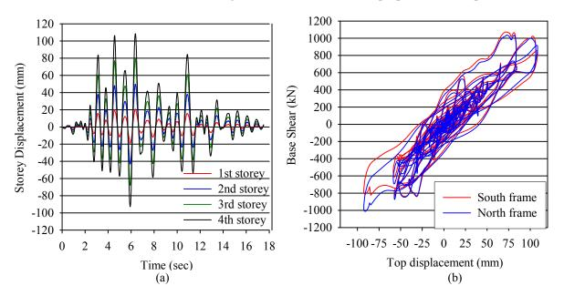
**Figure 3.2.** Experiment at 0.25 g acceleration (a) Variation of the storey displacements with time, (b) Base shear versus top storey displacement for the north and south frames
