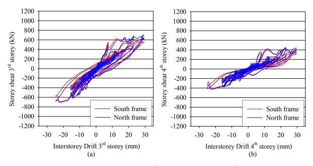
Figure 3.4. Experiment at 0.25 g acceleration (a) 3<sup>rd</sup> storey interstorey drift, (b) 4<sup>th</sup> storey interstorey drift
