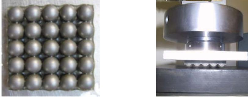
Fig. 2. Periodic surface and experimental set-up for the contact tests with the rubber block.
