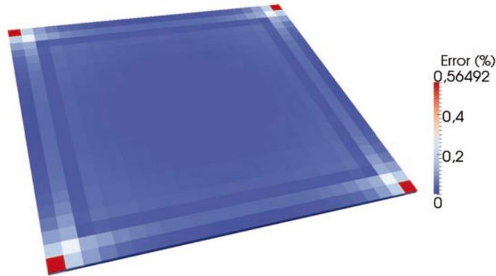
**FIGURE 3.** Relative error in strain energy density between 3D FEM and PGD based method
