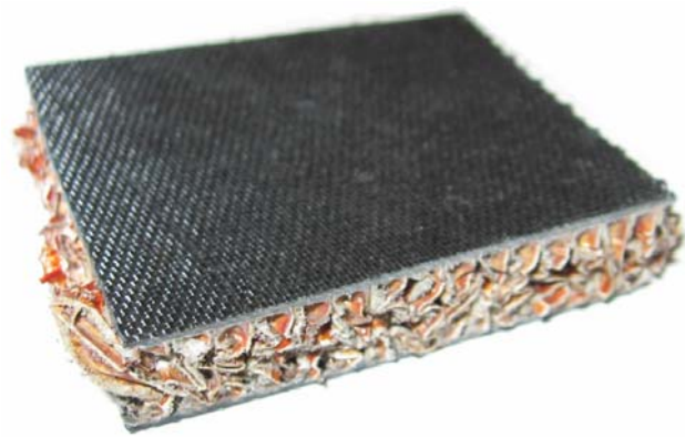
Figure 13: Sandwich specimen after crushing, Local buckling plies
