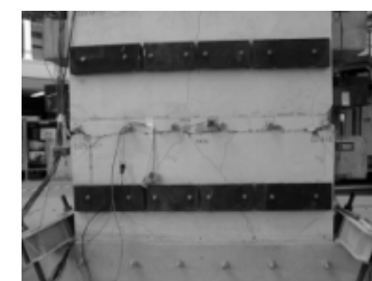
Figure 7. Comparison between test and analysis at failure: A) numerical vertical concrete strain contour at failure, B) crack pattern at the end of the test.
