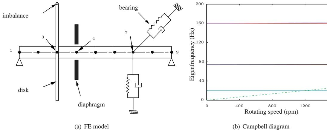
**Figure 4:** Model of shaft line
