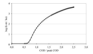
Figure 10: Evolution of logarithm of structural relative permeability with COD to peak COD ratio.
