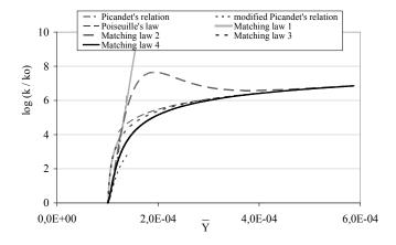
Figure 3. Logarithm of permeability evolution with state variable.
