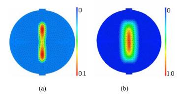
Figure 8: Damage distributions at (a) damage initiation and (b) at last loading step.
