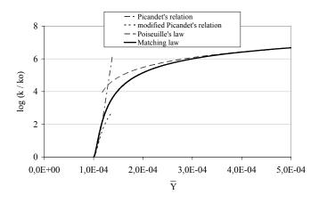
Figure 5. Logarithm of permeability evolution with state variable for the retained matching permeability law.
