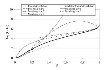
Figure 2. Logarithm of permeability evolution with damage.
