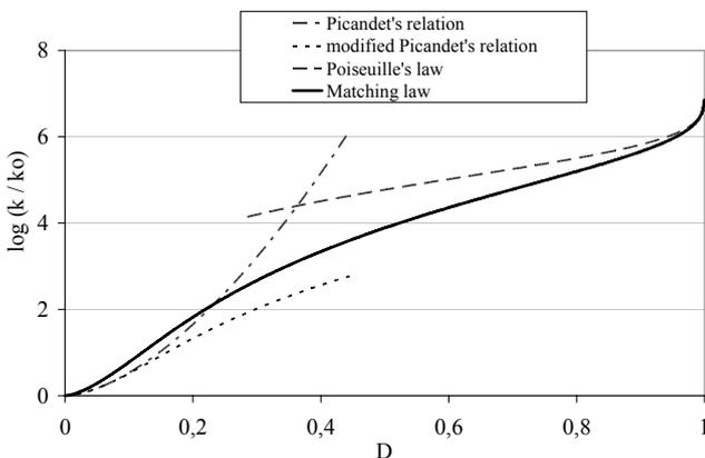
Figure 4. Logarithm of permeability evolution with damage for the retained matching permeability law.
