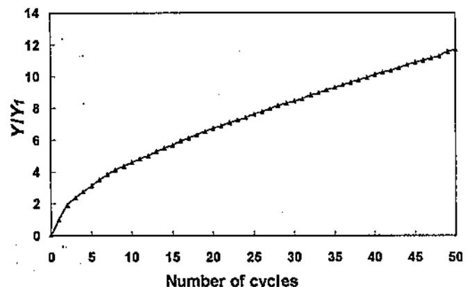
Figure 10. Normalized displacement – number of cycles relationship
