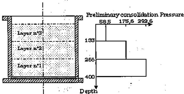
Figure 4. Preliminary consolidation pressure
