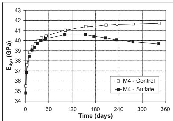
Figure 2. Elastic modulus of 4x4x16 cm<sup>3</sup> specimens.
