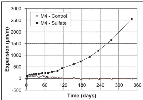
Figure 1. Expansion of 2x2x16 cm<sup>3</sup> specimens.
