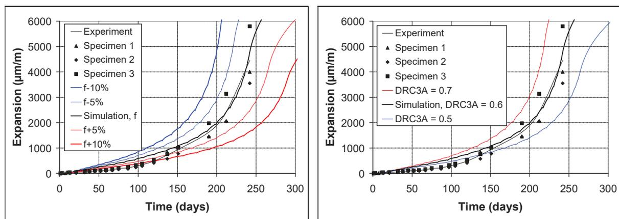
**Figure 4.** Sensitivity of simulated expansion to Fraction of capillary porosity that can be filled by expansive products  $f$  (left) and Degree of reaction of  $\text{C}_3\text{A}$   $\text{DRC}_{3\text{A}}$  (right).
