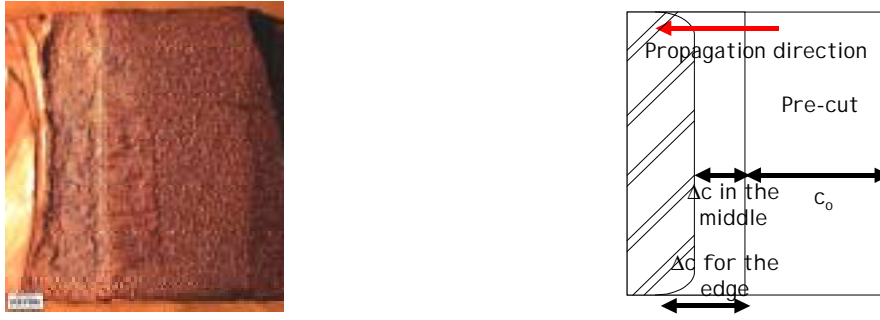
Figure 5 : shape of the crack front for a sample under plane strain conditions
