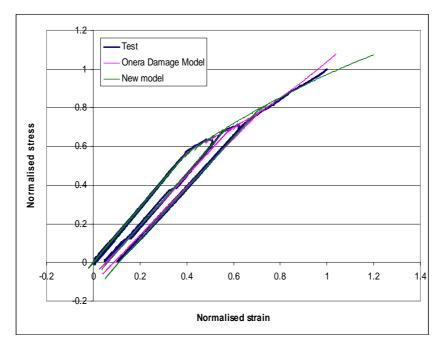
Figure 1: Load/unload test and simulation in the warp direction
