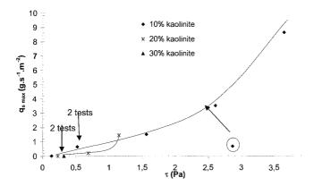
**Figure 5:** Maximum erosion rate v.s. hydraulic shear stress according to clay content  $(\sigma_3 = 100 \text{ kPa})$ .
