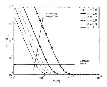
Figure 1: Evolution of the cohesion function  $1+F_{\text{c}}/F_{\text{W}}$  vs. particle diameter d for different porosity values.
