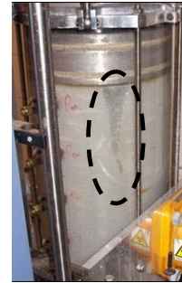
Figure 3: Downward progression of localized blowout
