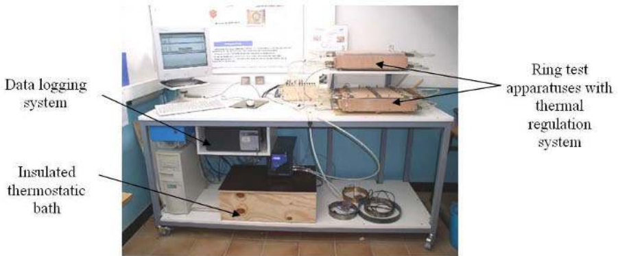
FIGURE 1. General view of the experimental device
