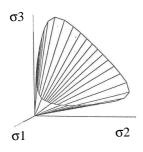
The soil behaviour is governed by the elasto-plastic Matsuoka-Nakaï criterion (Figure 12). It has been chosen because it is particularly suitable for granular materials as sand [Matsuoka, Nakai 1985]
