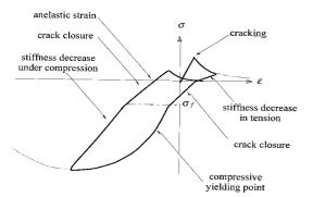
FIGURE 3. Tension-compression cycle
