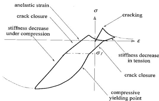
**FIGURE 3.** Tension-compression cycle
