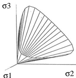
The soil behaviour is governed by the elasto-plastic Matsuoka-Nakai criterion (Figure 12). It has been chosen because it is particularly suitable for granular materials as sand [Matsuoka, Nakai 1985]
