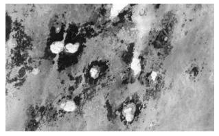
Figure 2. A Treated Specimen with Corrosion.
