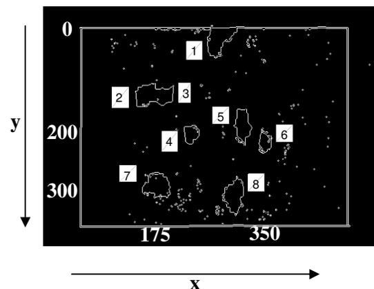
Figure 3. Detected Damage Regions in a Specimen.
